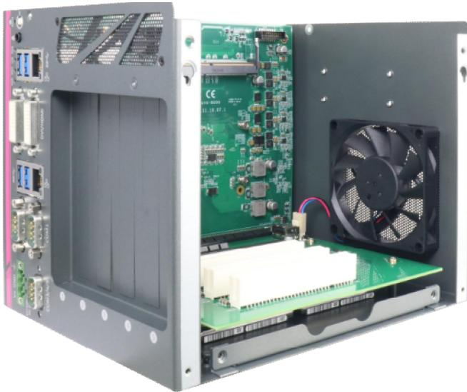
4. Fix the fan from outside using four F-head screws.
