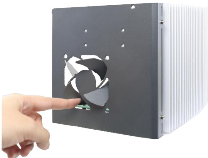
3. Align fixing holes of the fan to fixing holes on the back of chassis. Please make sure you have correct installation direction for fan as shown in the photo. The air flow must be from inside to outside. And plug the power connector of fan into the fan power receptacle on the backplane.
