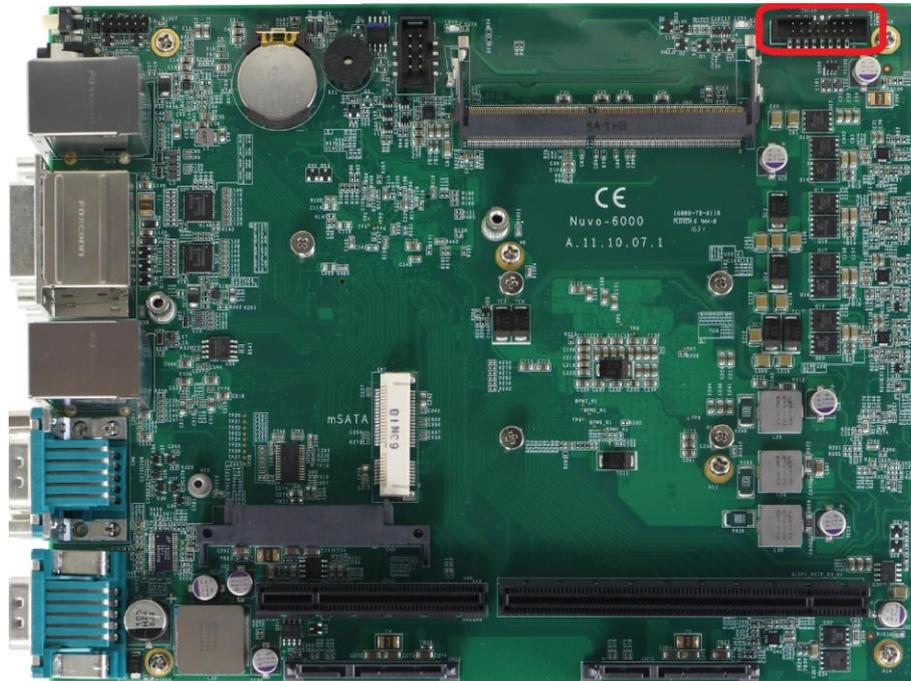
Nuvo-6000 provides additional two USB 2.0 ports internally via a 2x8 pins, 2.0mm pitch box header. The internal USB ports are designed to allow users attaching additional USB devices inside the chassis. To use the internal USB port, you shall need a dedicated box-header to USB cable. Please contact Neosys for further information.
