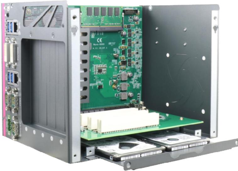
5. Secure the HDD/tray assembly to the chassis using two M3, F-head screws.
