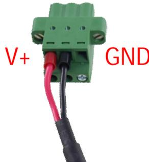
4. Insert the wires to correct contacts of pluggable terminal block and tighten clamping screws using a Philips screwdriver.
