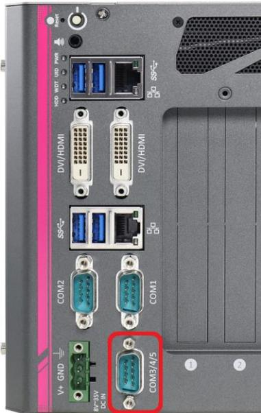
Nuvo-6000 provides totally five COM ports for communicating with external devices. These COM ports are implemented using industrial-grade ITE8786 Super IO chip (-40 to 85°C) and provide up to 115200 bps baud rate.
