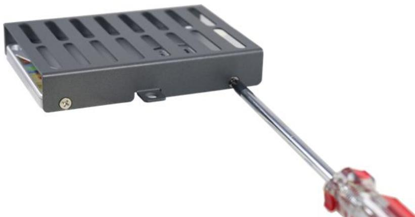
3. Gently insert the connector of SATA HDD/SSD into the SATA port #1 and make sure it's firmly contacted. Secure the HDD/bracket assembly to the SBC using two M3, P-head screws.
