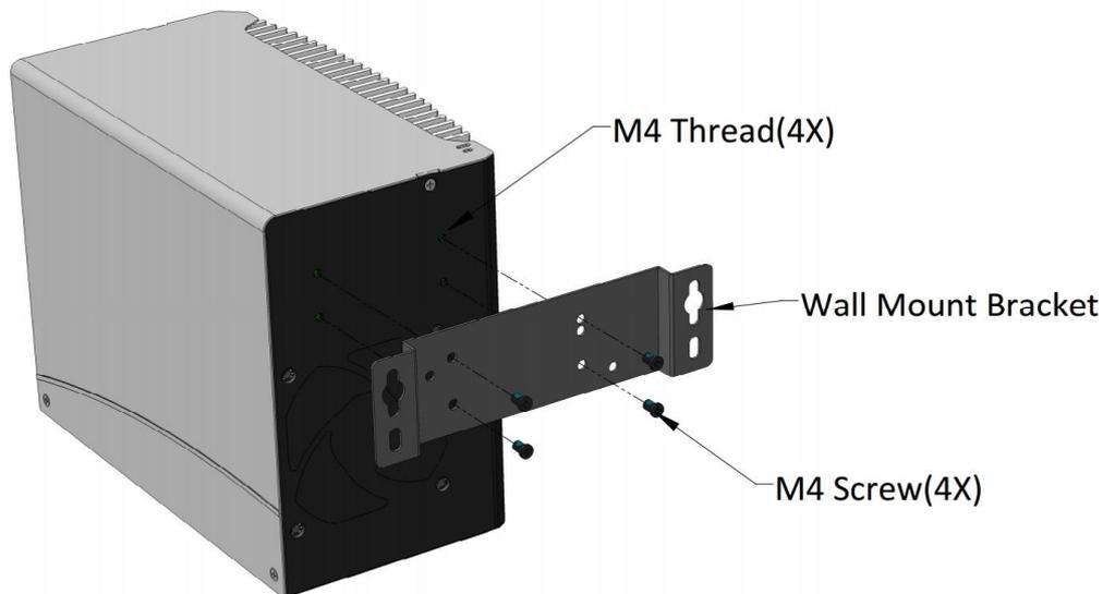
2. Fix Nuvo-6002 on the wall via the screw holes of the mounting bracket. You can also take advantage of the keyhole-shaped holes of the mounting bracket to suspend Nuvo-6002 on the Wall.
