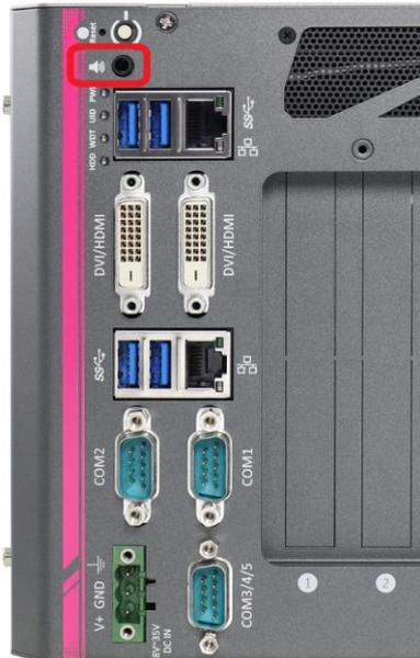
Nuvo-6000 provides audio function using Intel® High Definition Audio (built-in in H110 PCH) and Realtek ALC262 codec. There is an audio jack available on the front panel for speaker output. To utilize the audio function in Windows, you need to install corresponding drivers for both Intel® H110 PCH and Realtek ALC262 codec. Please refer to section 4.3 for information regarding driver installation.
