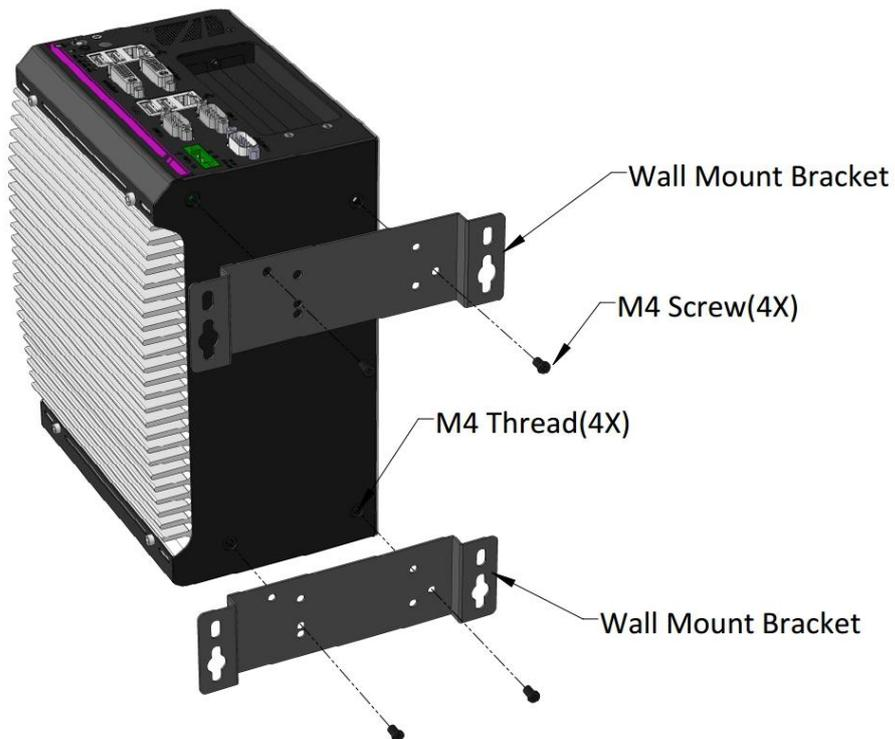
2. Fix Nuvo-6002 on a flat surface via the screw holes of two mounting brackets.
