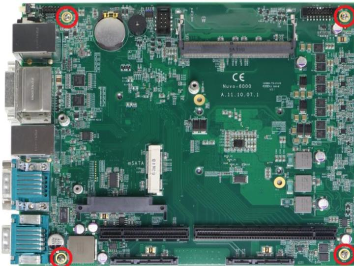
3. Gently lift the PCBA and separate it from the heat-sink.
