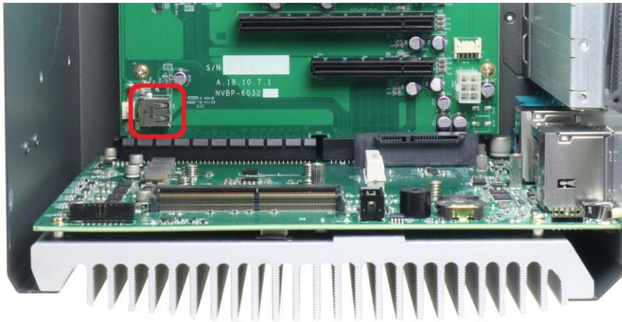
In addition to the USB header connector on the SBC, Nuvo-6000 offers another USB 2.0 Type-A port on the backplane. You can utilize this USB port to connect a USB protection dongle inside the chassis of Nuvo-6000 controller.
