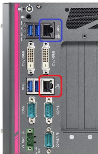
Nuvo-6000 series offers 2 GbE ports on its front panel. The GbE port marked in blue is implemented with Intel® I219-LM and port marked in red is implemented with Intel® I210-IT Gigabit Ethernet controllers. Each port has one dedicated PCI Express link to present maximal network performance. When plugging in the Ethernet cable, you can tell the Ethernet status and speed from the LED indicators on the RJ45 connector as following:
