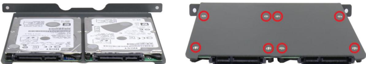
4. Align the HDD tray with guided nuts on the bottom of chassis and slide it into the chassis till SATA HDD drives are firmly attached to the connectors on SBC.
