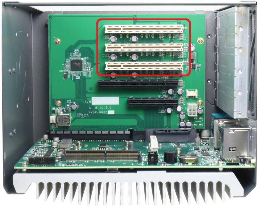
Nuvo-6032 provides three PCI slots, which support 5V, 32-bit/33MHz PCI bus, to accommodate PCI add-on cards. The maximum allowable length of a add-on card to be installed into Nuvo-6000 is varied depending on whether the optional fan is installed. Please refer the following table to understand the restriction of dimension for add-on cards. For information of installing PCI cards, please refer to section 3.6 for detail.
