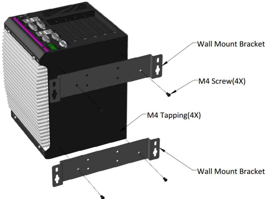
2. Fix Nuvo-6032 on a flat surface via the screw holes of two mounting brackets.
