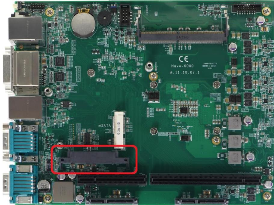
Nuvo-6000 provides totally three SATA ports. Nuvo-6032 can accommodate three 2.5" SATA hard drives and Nuvo-6002 can only accommodate one due the restriction of chassis space.
