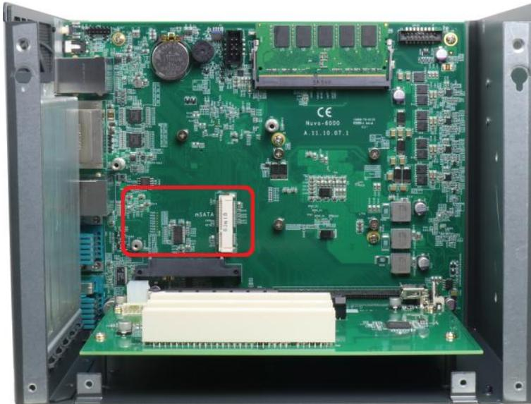
2. Tilt the mSATA SSD module and insert it into the mSATA socket. And fix the module with one M2.5 P-head screw.
