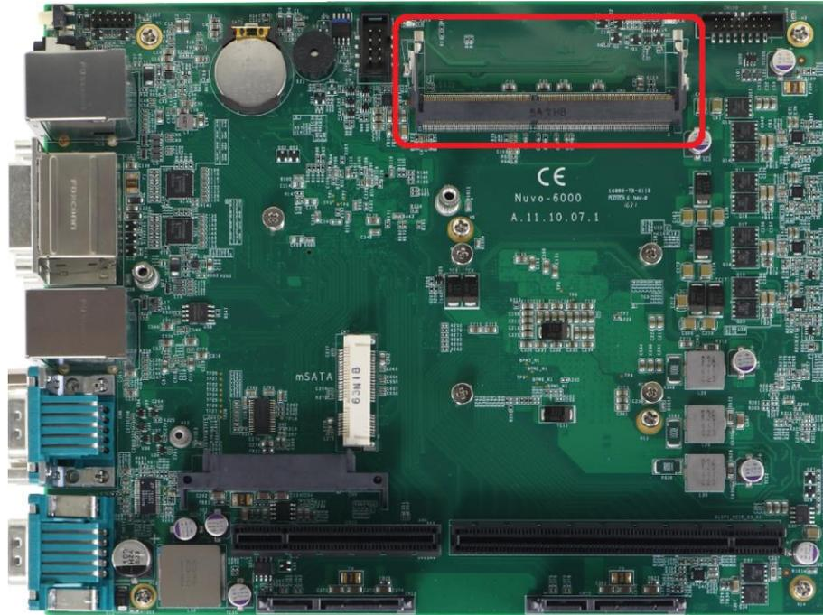
Nuvo-6000 series provides one 260-pin, SODIMM socket for installing DDR4 memory module. It supports maximal 16GB capacity by installing one 16GB DDR4 2133 MHz SODIMM modules. For information of installing DDR4 memory modules, please refer to section 3.3 for details.
