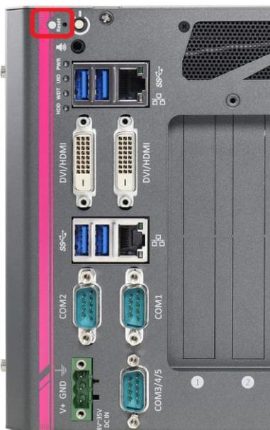
The reset button is used to manually reset the system in case of any abnormal condition. To avoid unexpected operation, the reset button is hidden behind the front panel. You need to use a pin-like object to push the reset button.
