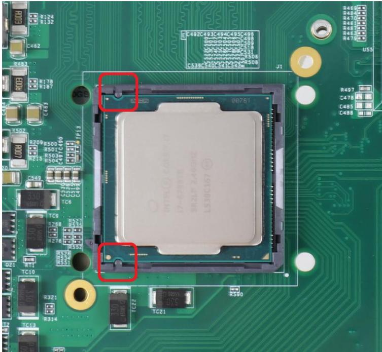
6. Get the CPU retaining bracket from the accessory box and place it on the top of CPU. The CPU retaining bracket must be screwed from the opposite side. Please hold the CPU and bracket firmly while turning the PCBA upside down, and secure the CPU retaining bracket with two M3 P-head screws.
