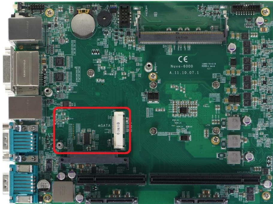
Nuvo-6000 provides a mSATA port to accommodate mSATA flash disk module. mSATA is a solid-state storage device with SATA interface and is very reliable for harsh environments with intense vibration/shock. The system recognizes mSATA as a native storage device and accordingly you can install any operating system in the mSATA module, such as Windows 7, Windows 8, Windows 10, Linux and etc.
