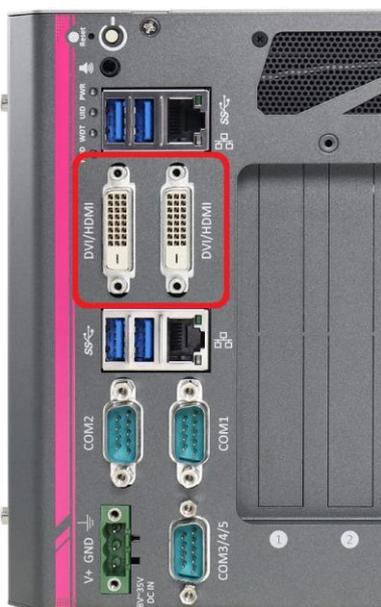
Nuvo-6000 series has two DVI-D connectors on its front panel to support dual independent display outputs. DVI/HDMI transmits graphics data in digital format and therefore can deliver better image quality at high resolution. The DVI/HDMI connectors can either output DVI signals or HDMI signals depending on the display device connected. It supports up to 1920 x 1200 resolution. You can use a DVI to HDMI cable to connect a HDMI display device.
