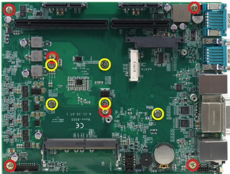
3. Gently lift the SBC from the heat-sink. The CPU and CPU retaining bracket shall stay with the heat-sink.
