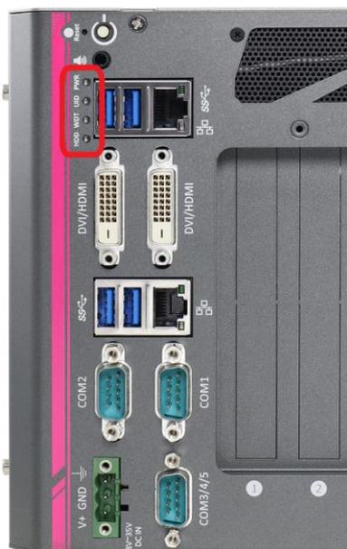
There are four LED indicators on the front panel: PWR, UID, WDT and HDD. The descriptions of these three LED are listed in the following table.
