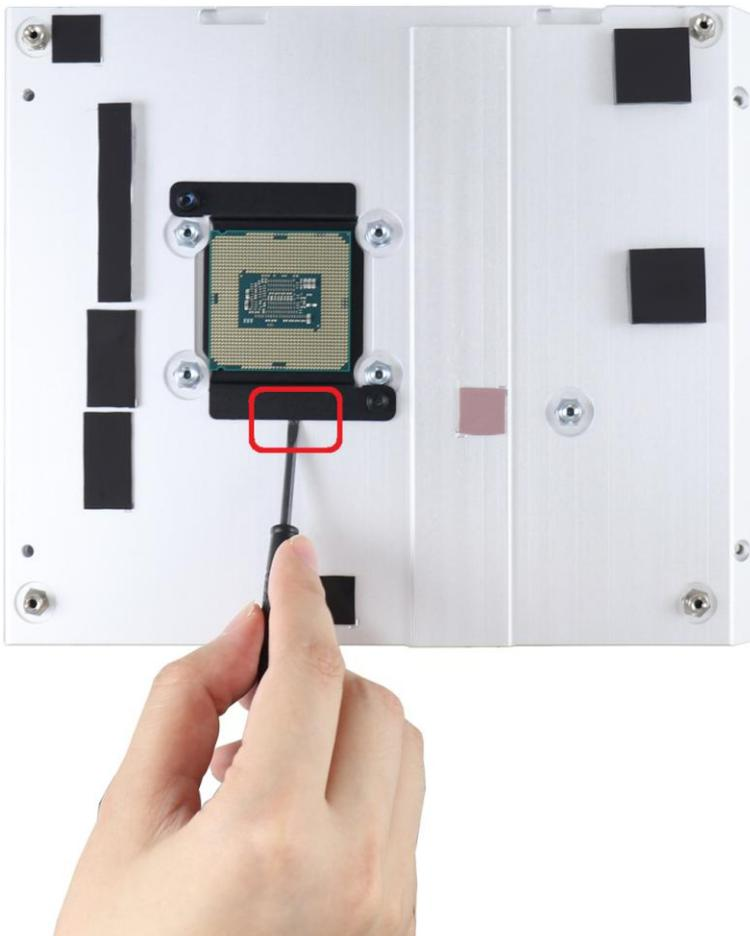
5. Check the condition of thermal pads on the heat-sink, especially the thermal pad for CPU. If it's broken, please replace it with a new one.
