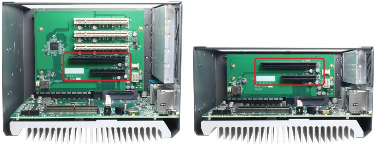
Both Nuvo-6032 and Nuvo-6002 provide one x8 and one x16 PCI Express slot. The x8 slot is running at Gen2, 4-lanes PCIe signals and can deliver up to 2 GB/s bandwidth. The x16 slot is running at Gen3, 16-lanes PCIe signals and is suitable for both graphics card and I/O card installation.
