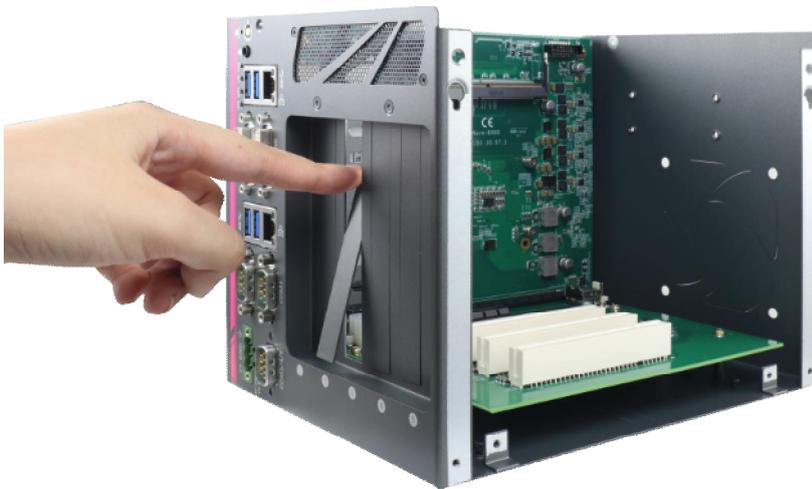
2. Install your add-on card into the PCI/PCIe slot. Make sure the “golden finger” connector is firmly contacted with PCI/PCIe connector and the faceplate of the add-on card is well inserted to the groove underneath.
