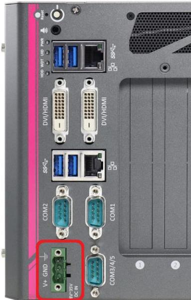
Nuvo-6000 series allows a wide range of DC power input from 8 to 35V via a 3-pin pluggable terminal block, which is fit for field usage where DC power is usually provided. And the screw clamping connection of the terminal block gives a very reliable way of wiring DC power. For detail information of supplying DC power via pluggable terminal block, please refer to section 3.9.
