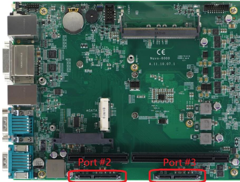
Nuvo-6000 provides totally three SATA ports. Nuvo-6032 can accommodate three 2.5" SATA hard drives and Nuvo-6002 can only accommodate one due the restriction of chassis size.
