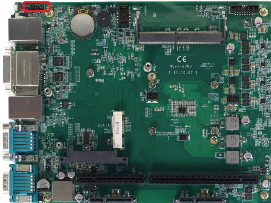
For an application which places Nuvo-6000 inside a cabinet, it's useful to output the system status to external LED indicators so that users can check how the system's running. Nuvo-6000 provides a 2x6, 2.0mm pitch pin header to output system status such as power, HDD, watchdog timer, and control system on/off remotely.
