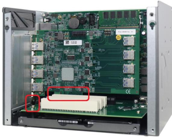
3. Fix the PCI/PCIe add-on card using the M3, PW-head screw.
