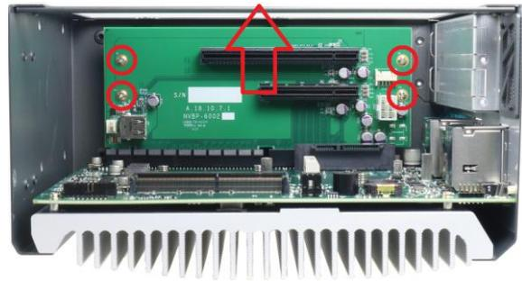
3. Remove two hex screws near COM3/4/5 connector.
