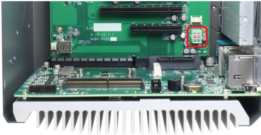
Some high-watt add-on cards require additional 12V input. Nuvo-6000 offers a 6-pin PCIe power connector on its backplane to provide up to 8A rated current. This can be useful if you want to power a PCI Express graphics card with up to 90W TDP.
