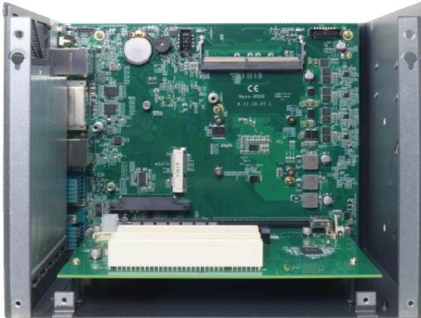
2. Tile the SODIMM module and insert it to the SODIMM socket. As it's firmly contacted with socket connectors, press it down until the clamps of the socket snap into the latching position of SODIMM module.
