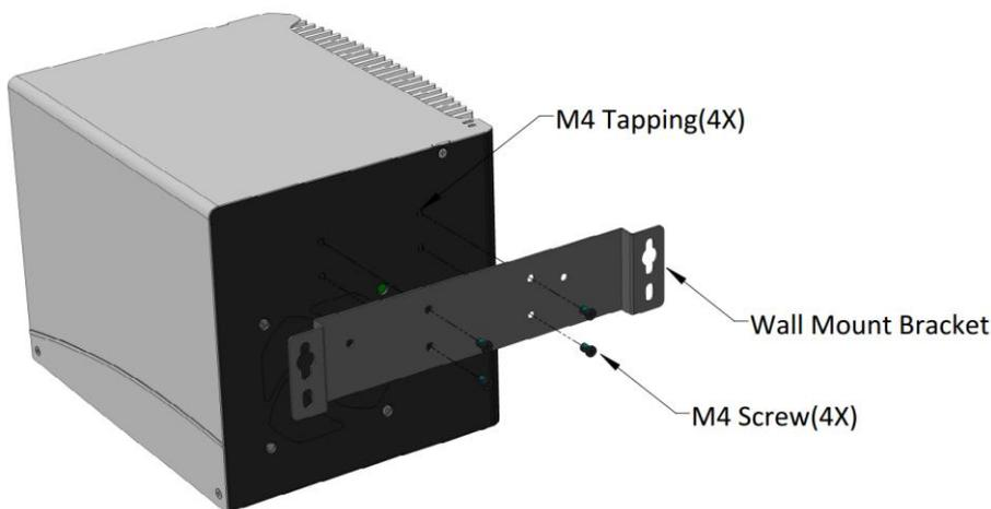
2. Fix Nuvo-6032 on the wall via the screw holes of the mounting bracket. You can also take advantage of the keyhole-shaped holes of the mounting bracket to suspend Nuvo-6032 on the Wall.
